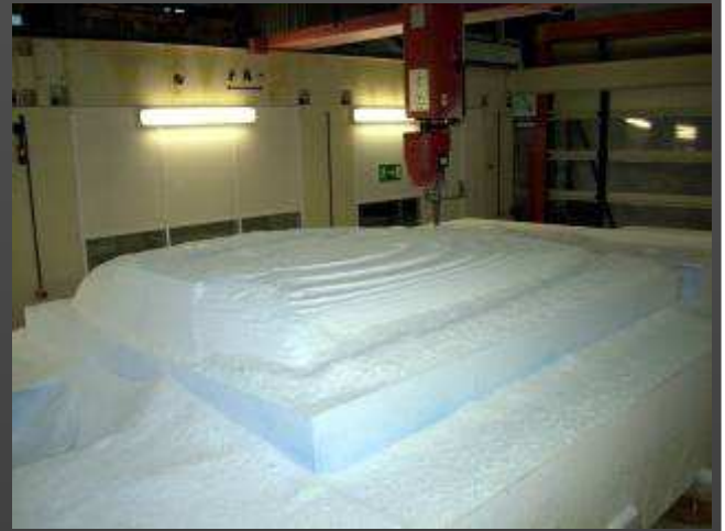
Machining polystyrene block
