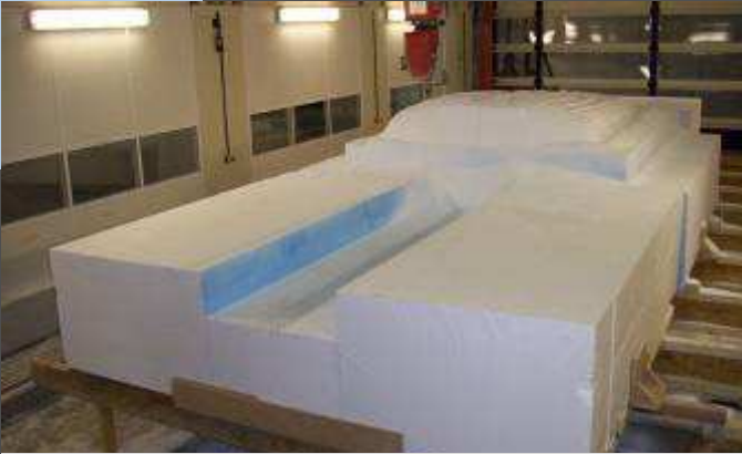
Machining polystyrene block
