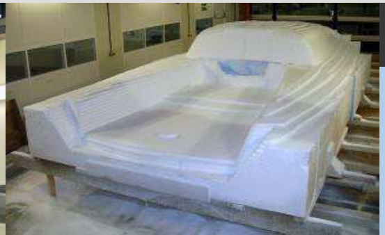
Block of polystyrene assembled on a metallic frame assuring the stability .
