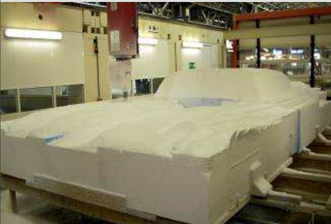
Block of polystyrene assembled on a metallic frame assuring the stability .
