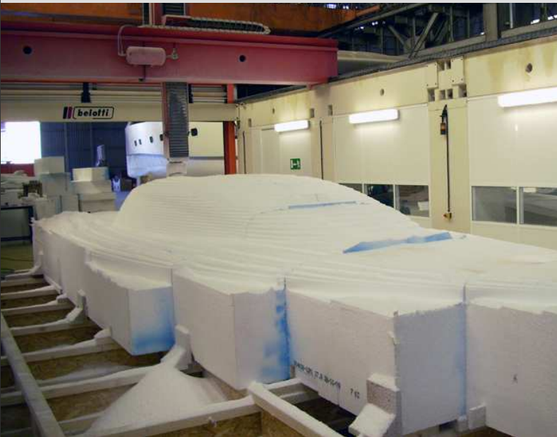
Block of polystyrene assembled on a metallic frame assuring the stability .
